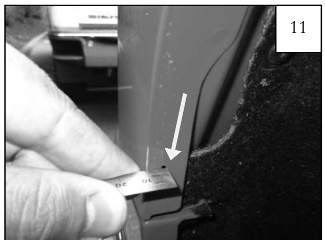
Remove the flare. At the marked location made in Step 9, measure inward 10mm from the edge of the fender. These are the marks to be drilled. Note: Marks at 10mm may be on either side of the first mark.
