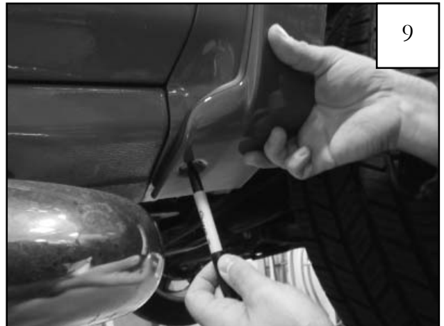
While still holding front of the flare firmly on the fender. Make sure front of flare is aligned with bumper style line. Using a grease pencil, mark the bottom fastener location using flare as guide.
