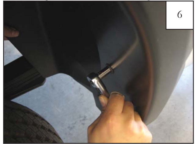
Holding flare in position on fender, reinstall screws removed in Step 5. Do not tighten. (An awl may be used to align the threaded clip with holes in flare and fender lip) Note: Make sure screws engage in splash shield.
