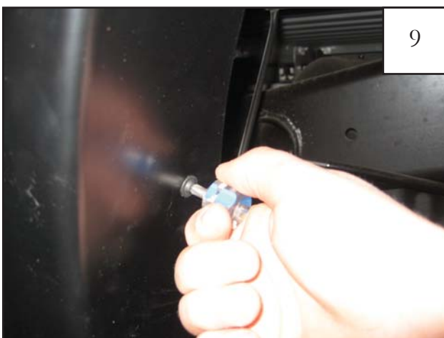
Using #2 Phillips Screwdriver, insert a supplied Truss-Head Screw through existing holes in flare and into holes in clips (4 places).
