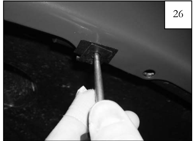
Using an awl or similar pointed tool, poke a hole through plastic tab using the speed clip hole as a guide.
