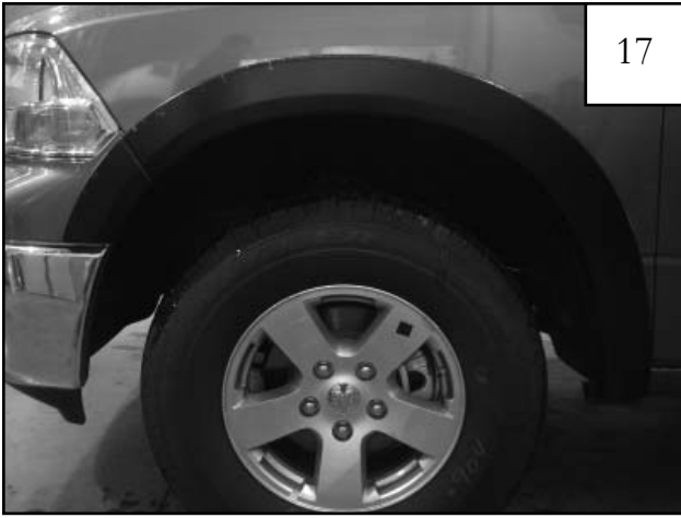
METAL BUMPER ONLY: Completed front flare installation.
