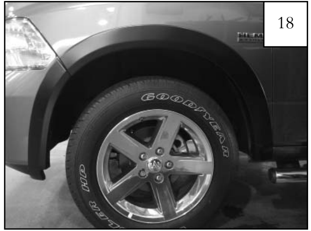
PLASTIC BUMPER ONLY: Completed front flare installation.
