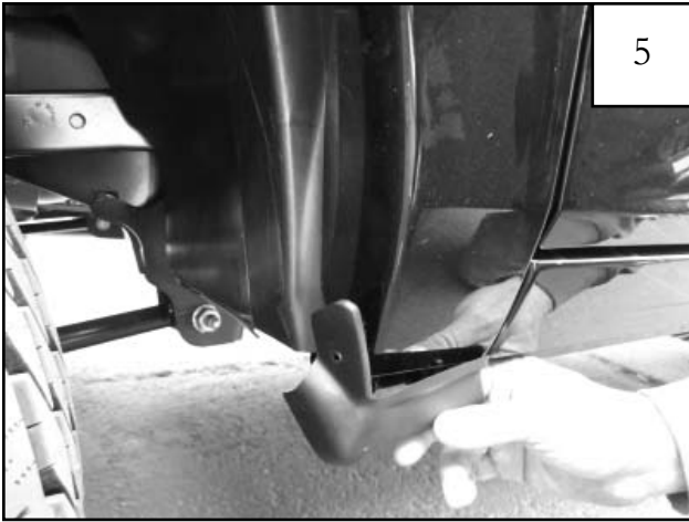
2011-Up Models Only (Optional): If you encounter a fit problem, remove inner pieces at front and rear of wheel well.
