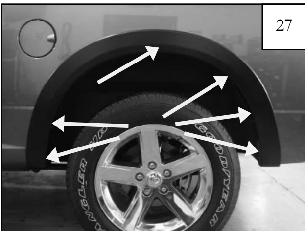
Supplied screw locations. Install one supplied screw at the top of flare first for easier installation. See step 28.
