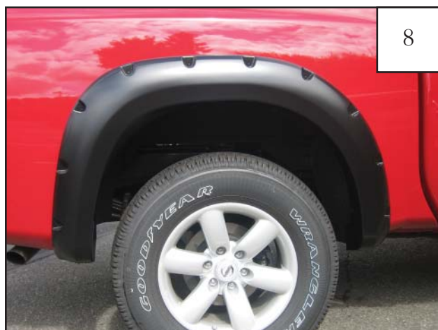
Passenger Side Flare: Completed rear flare installation.
