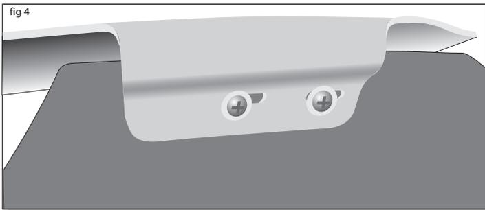
**7** Adhere the center of the Hood Protector to the hood by grasping the hanging red backing on the adhesive strip and removing it from the adhesive. Apply firm pressure to set into place.
