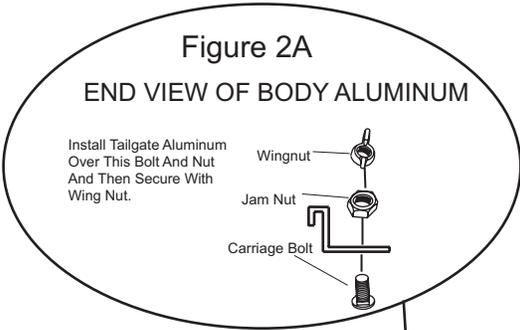
Drill 5/32" Hole Through Pre-Punched Hole in Alum. After Alum is Bolted Down
