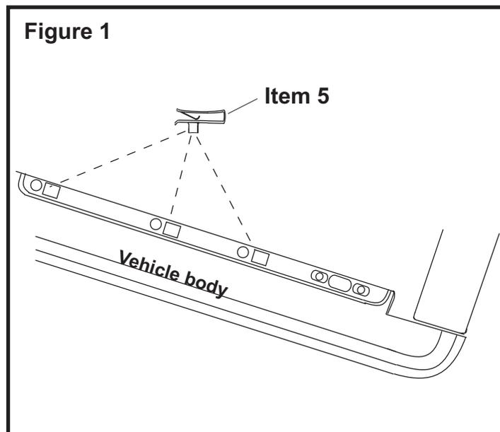
rear of the rear body aluminum. Now tighten both bolts using the 1/2" wrench or socket. Using the pre-punched small hole in the rear of the rear body aluminum as a guide, drill a 5/32" hole into the body. See Figure 2. Install the sheet metal screw (item #10) through the pre-punched hole and the nylon spacer (item #15) and into hole drilled in body. Do not fully tighten screw. Now loosen other two bolts tightened earlier.
